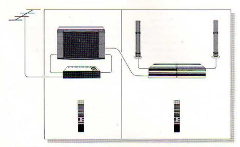
Situation 2: The video and the audio systems placed far away from each other, e.g. in separate rooms, so that the commands from the Beolink 1000 remote control unit can be received only by either of the systems at a time.
