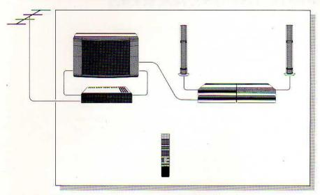
Situation 1: The video and the audio systems placed close together so that the commands from the Beolink 1000 remote control unit can be received by both systems simultaneously.
